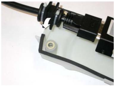
Image 3-4 Insert connection into housing
